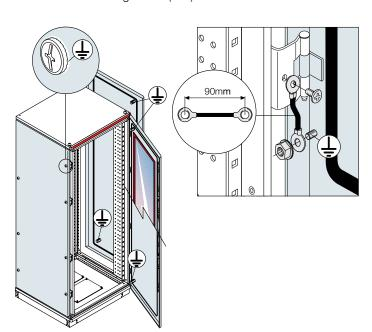
The special shape of the hinge allows connection even using a traditional copper braid.
