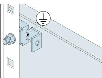
The blind door, side panels and rear panels are fitted with copper M6captive screws. Panel earthing is obtained thanks to the fixing screws.
